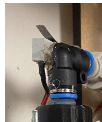
Figure 22 Limit switch attached to gripper for homing lead screw
