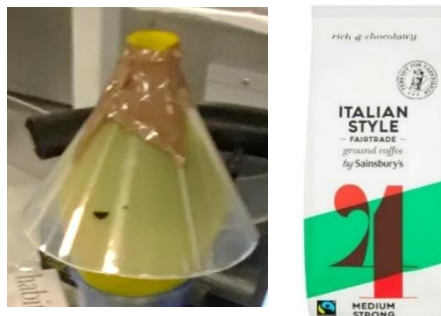
Figure 8 (Left) Balloon gripper proof of concept (named Esteban) and (right) the coffee grounds used in the balloon
