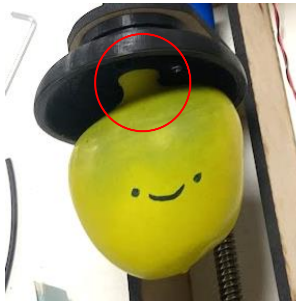
Figure 31 Balloon neck supports the weight of the balloon
